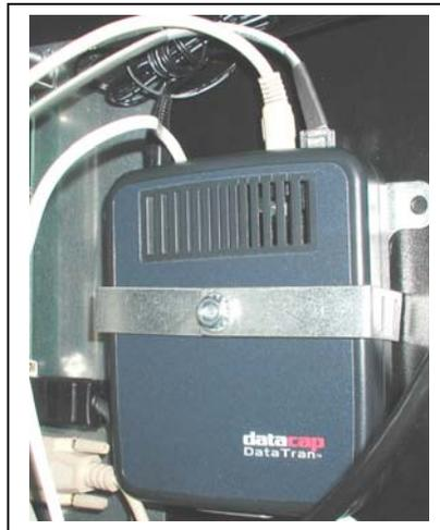
The credit card terminal is comprised of a card reader and a modem. The modem shown here is the DataTran 162SL. This is the box that connects to the phone line.
